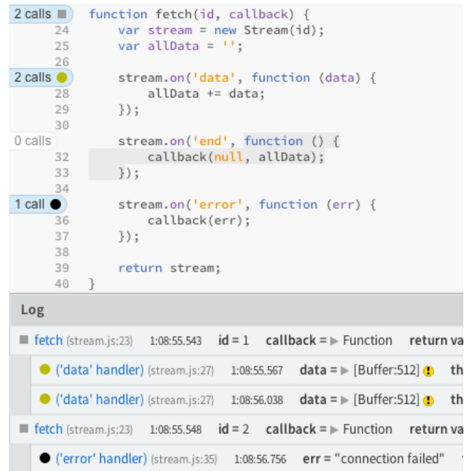
Figure 1. Theseus shows call counts for every function, and an asynchronous call tree allows the user to see how functions interact. In the log above, users can see which call to fetch corresponds to the failure without adding any debugging-specific code or instrumentation.
